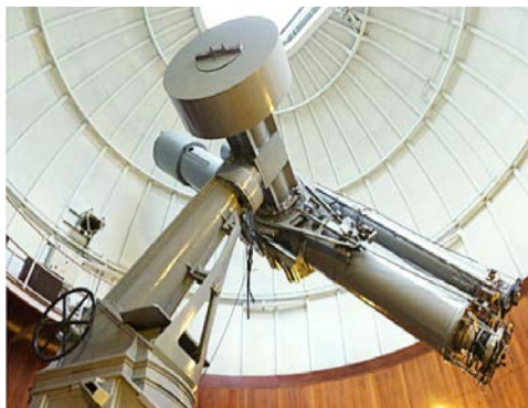
26" Thompson Refractor Employs a 26" dia. Lens to collect the light
